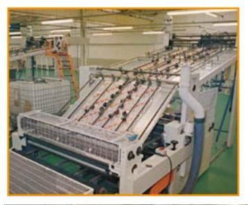
Gluing of a pre-printed solid board sheet or a web onto single-face corrugated or compact board
